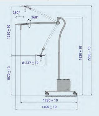
The mobile examination light EMALED 202 M with a battery back-up can be used without power connection up to 24 hours. The high illumination and excellent lightning quality makes this mobile surgical light a good allrounder in multiple fields.
